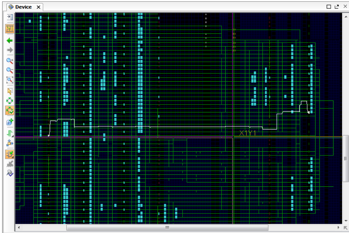
Figure 9: Displaying the Device Routing
