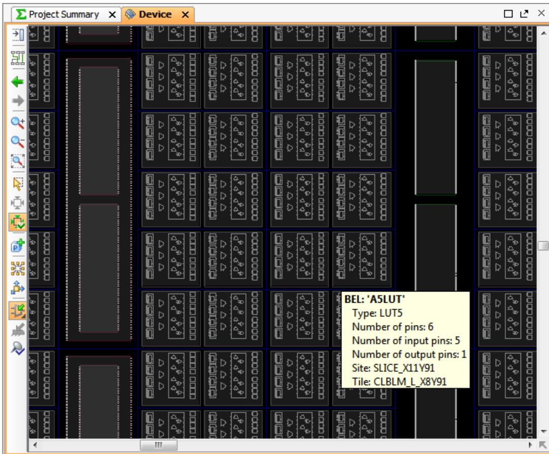
Figure 7: Viewing Sites, Slices and BELs in the Device window
