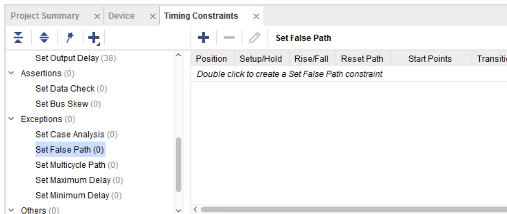
Figure 17: Set False Path Section in the Constraints Editor
