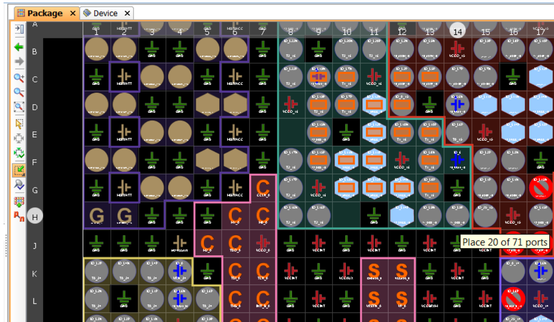
Figure 3-26: I/O Ports Placed in an Area
