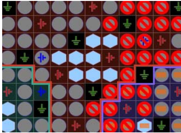
Figure 3-22: Prohibits on Package Pins
