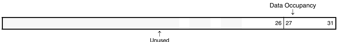
Figure 6: ADCout Data FIFO Occupancy Register (C_DACIN_WIDTH = 9)
