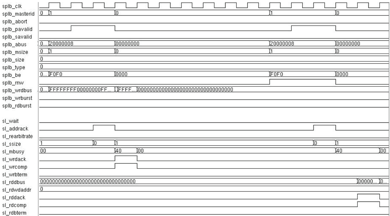
Figure 16: Single Write and Read Transfers to PLBV46 to AXI Bridge Register (DGIE)
