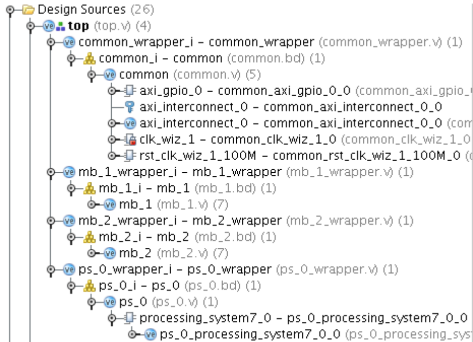
Figure 4–1: Example Design with multiple block design instances in the active top design
