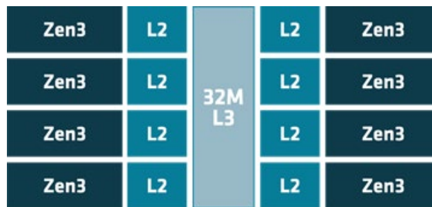
Figure 1 AMD EPYC 7003 Processor L3 Cache layout
