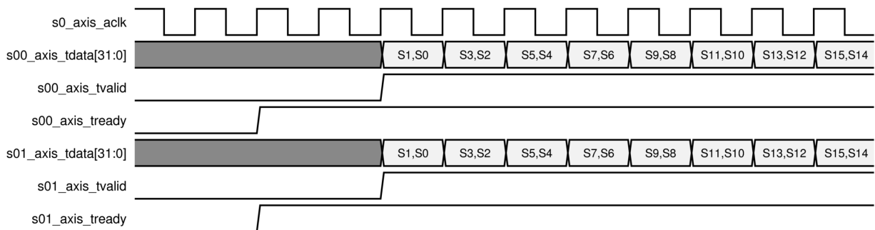
Figure 81: Two RF-DACs with Real Data on Separate Interfaces at 250 MHz
